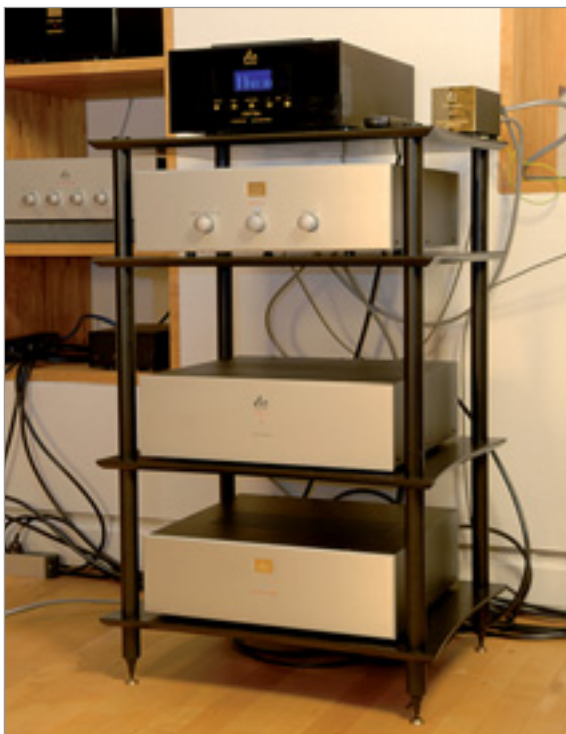
From top to bottom: MC step up transformer behind the CD transport, preamplifier, D/A converter, valve power supply
