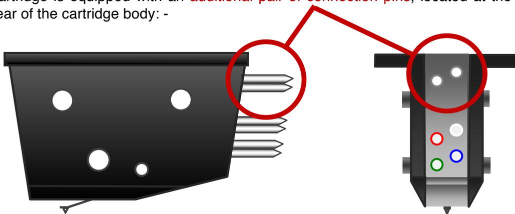
To connect these pins to the external power supply unit, an additional pair of internal (or external) arm wires and a two core / twisted pair external arm cable of suitable length (to reach the external power supply unit) will be required.
