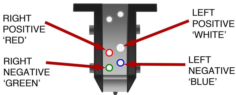
As the IO Ltd is a field coil design, it requires a DC voltage to generate the internal magnetic field. To receive this voltage from the external power supply unit, the cartridge is equipped with an **additional pair of connection pins**, located at the top / rear of the cartridge body: -
