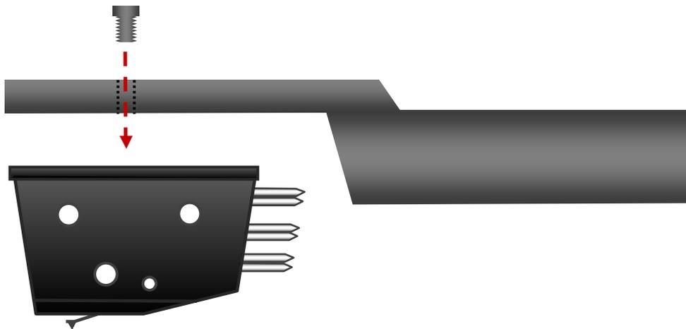
Once the cartridge is in place, set the correct tracking weight. Do this BEFORE the final adjustments are made for cartridge alignment, as this will help to ensure the cantilever is not damaged due to excessive tracking force. Once final alignment adjustments have been made, it will be necessary to check the tracking weight again, as any movement of the cartridge body will change the tracking weight.
