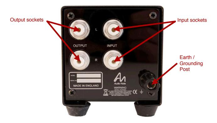
Once located, connect the AN-S8 between your turntable and phonostage input. Connect your tonearm / turntable output cables to the input sockets on the AN-S8, and the output sockets of the AN-S8 to your MM phonostage input. It is important to use good quality, shielded interconnects for all turntable connections; this will help to minimize any noise or hum problems.
