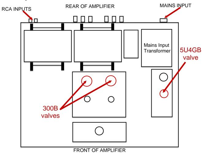
In the above drawing, the positions of the valves are marked in RED.
