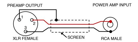
CABLE CONFIGURATION FOR XLR BALANCED PREAMP
