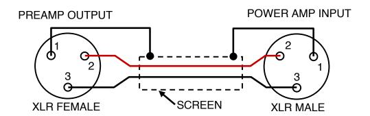
CONVENTIONAL: SCREEN CONNECTED AT BOTH ENDS
