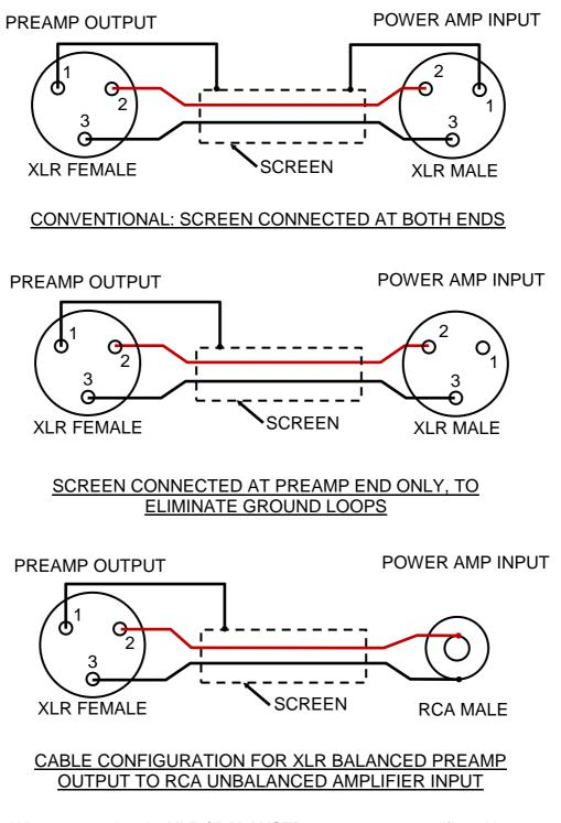
When connecting the XLR / BALANCED outputs to an amplifier with an RCA / Single Ended input, the switch must be set to the 'SINGLE ENDED' position.
