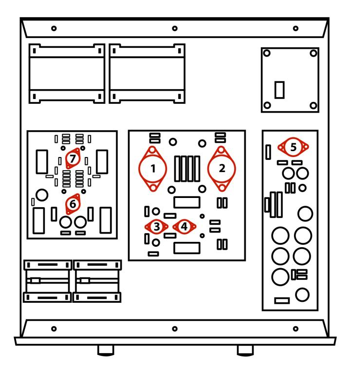
VALVE 1; 300B VALVE 2; 300B VALVE 3; 5687 VALVE 4; ECC82 VALVE 5; 5U4GB VALVE 6; ECC88 VALVE 7; ECC83
